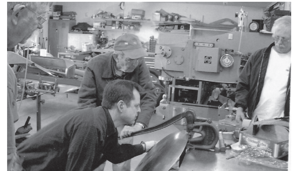
John Sweeney helps Duanne Luckow punch holes in the newly fabricated spare wheel well.
