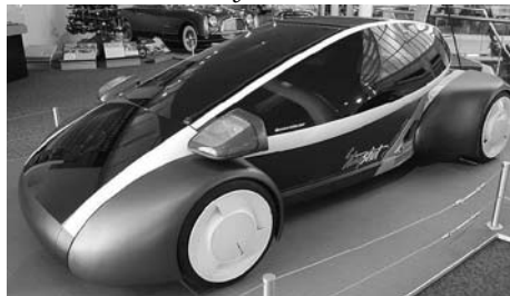
1988 Plymouth Slingshot: The Slingshot was targeted at the young people of the 1990s. It was designed as part of a series of three sports cars from Chrysler (along with the "Big Shot" and "Hot Shot"). The Slingshot features a mid-mounted, 2.2L DOHC inline-four engine, with twin cams, 16 valves, and an intercooled turbocharger.
