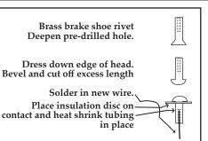
up against the disc and contact head and heat shrink it in place. This keeps the contact head from protruding when the light bulb is removed and prevents and possibility of electrical shorts. You now have a good connection that may even be better than the original.
