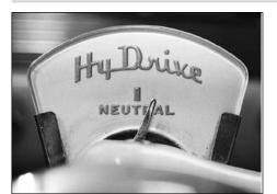
Cars equipped with Hy-Drive wouldn't start unless the transmission was in neutral, and that's the only position marked on the selector quadrant.
